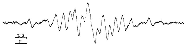
Figure 2. ESR spectra of radicals produced by photolysis of \text{H}_2\text{O}_2 in ethyl ether-propylene after 40 min of irradiation at -80^\circ .
